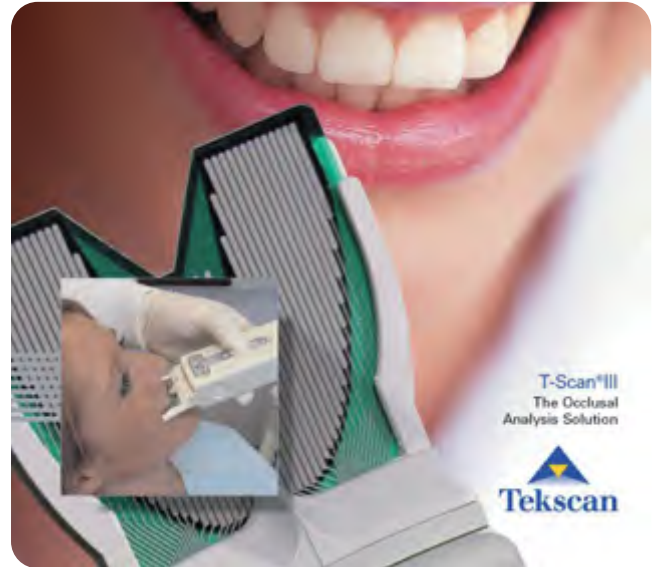
Figure 1.21. The T-Scan III is a computerized device that allows precise mapping of occlusal forces during the entire timing of closure from first contact to maximum intercuspation.
